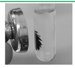
FastWoRX-M is a hydrophobic and magnetic black powder that absorbs most organics. It can easily and quickly be separated - along with the absorbed organics — from the aqueous phase by a magnet or a simple filtration. Using an electromagnet allows easy collection and release of the powder, enabling many automation possibilities.
